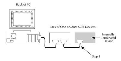
2. Disconnect the end of that cable from the internally terminated device. Do not disconnect the other end of the cable.
